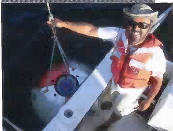
Deployment of an Acoustic Doppler Current Profiler (ADCP) in Coastal Waters.
