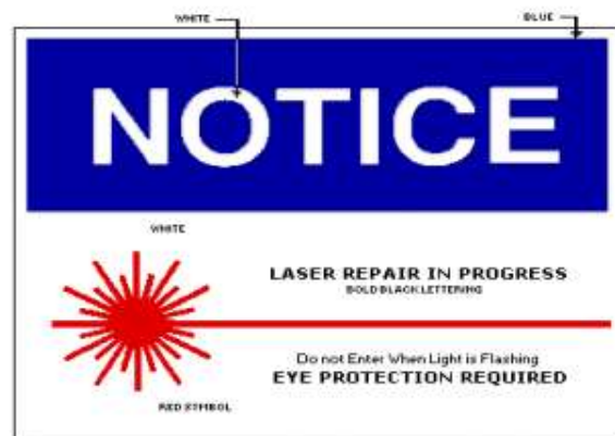
Figure 2, Temporary Signage for Maintenance of Embedded Lasers
