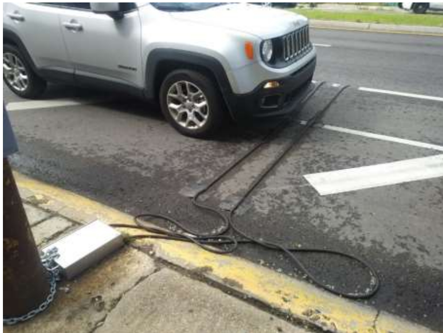
Figure 1 Tulane Avenue count equipment configuration, inbound
