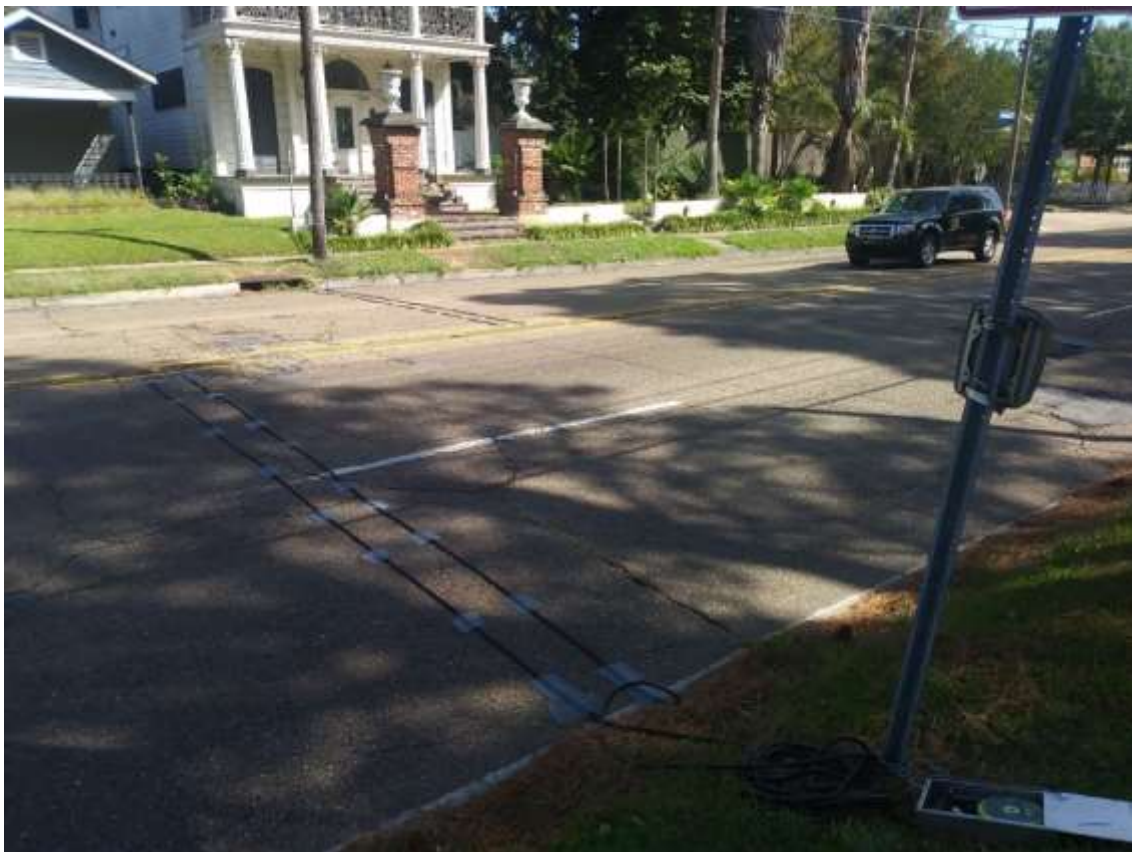
Figure 18 Government Street count sensor configuration, inbound and outbound
