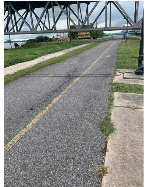
Figure 1 Infrared sensor and pneumatic tube counters collecting usage pattern data on Baton Rouge Mississippi River Levee Trail Photo Credit: Tara Tolford
