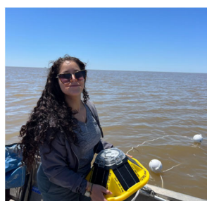
Undergraduate researcher Victoria Sanchez deploying a wave data buoy in the Wax Lake Delta, Atchafalaya Bay, Louisiana. These buoys broadcast live real-time data hourly and can be publicly viewed and downloaded here: https://spotters.sofarocan.com/?spotter-filter=SPOT-30807C
