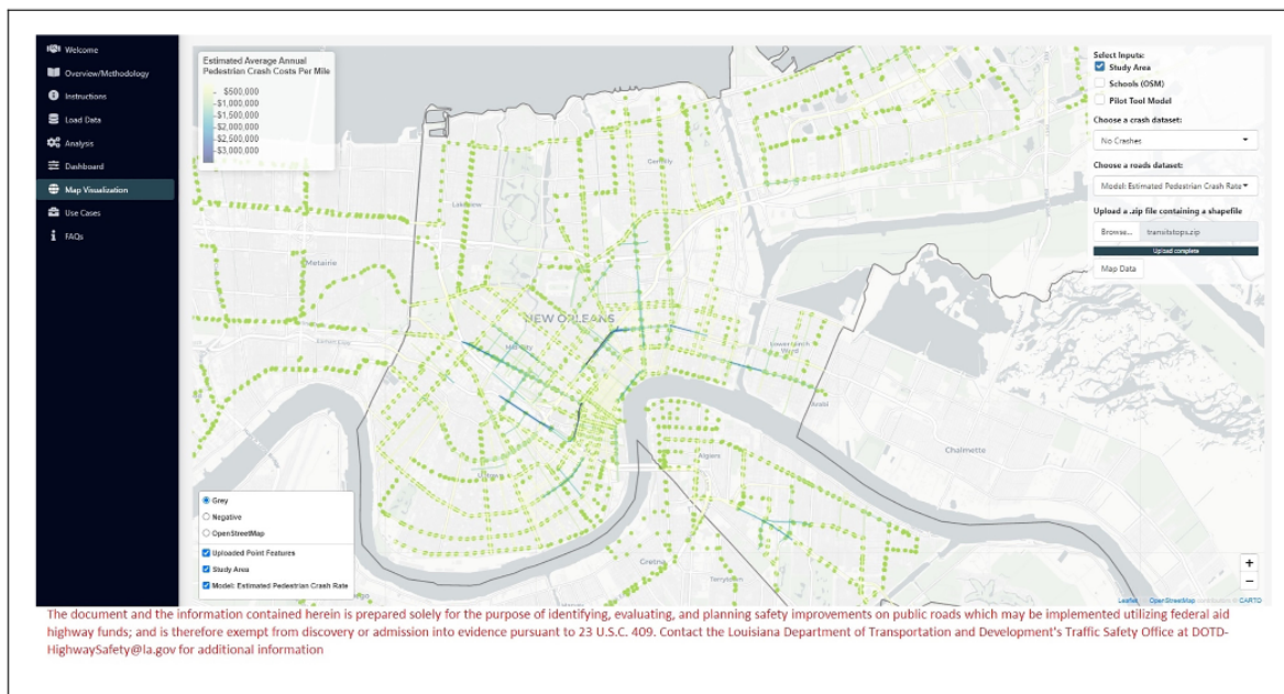
Figure 5. Map visualizer showing outputs for pedestrian risk model, overlaid with transit stop point features.
