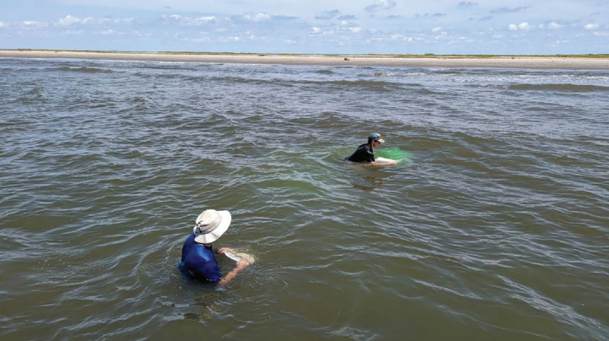
Researchers release fluorescent sand pellets off the shoreline in Lafourche Parish, Louisiana.
