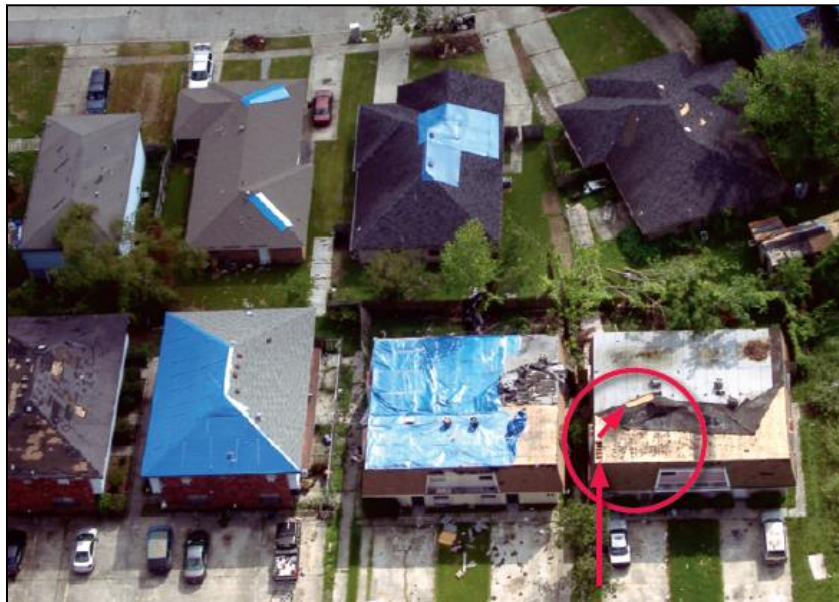
Figure 6-8 Hurricane Katrina: Typical Wind Damage to Residential Structures
