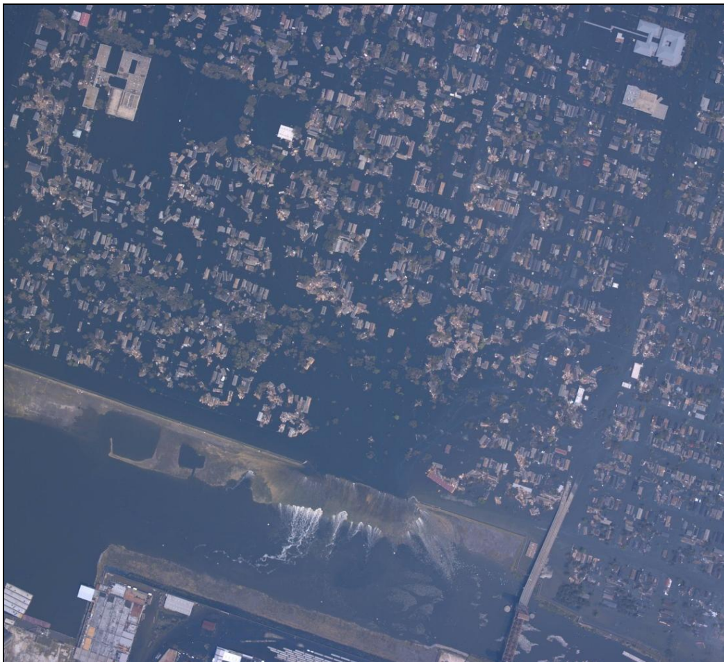
Figure 6-31 Industrial Canal; South Breach at the Lower Ninth Ward on August 31, 2005 (Source; NOAA – August 31, 2005)
